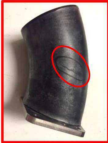
Picture 3 : Weld line NG
